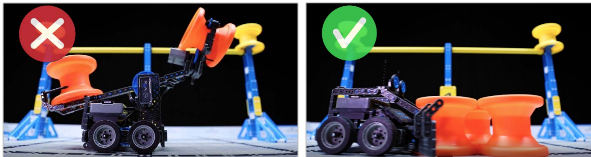
Figure 8 (left) – Example of a Robot holding more than one Hub off of the Floor at once, in violation of <G17>. Figure 9 (right) – Example of a Robot pushing multiple Hubs that remain in contact with the Floor. This is permitted within <G17>.
